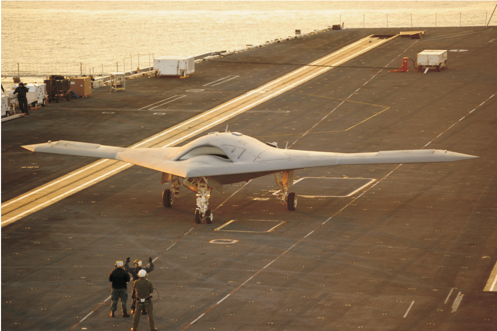
The X-47B Unmanned Combat Air Vehicle (UCAV), developed by Northrop Grumman in cooperation with DARPA, is popularly referred to as “semiautonomous”. (Courtesy of Northrop Grumman)
