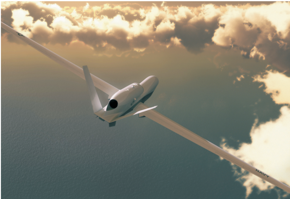
The “TRITON” – under development by Northrop Grumman for the US Navy to be part of the Broad Area Maritime Surveillance (BAMS) programme – is an advanced intelligence, surveillance and reconnaissance missions system, which may operate under control or autonomously. (Courtesy of Northrop Grumman)
