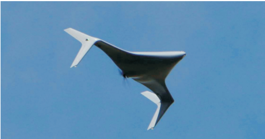
The “BAT” by Northrop Grumman (formerly “KillerBee” by Raytheon) is a medium-altitude drone able to operate at extended ranges with a variety of sensors and payloads, and probably at least electronic warfare capabilities. (Courtesy of Northrop Grumman)
