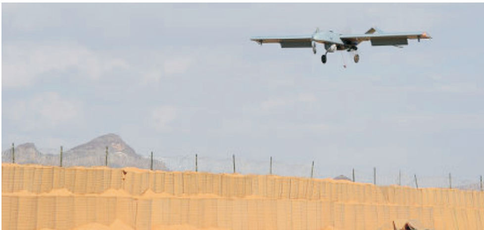
Shadow Unmanned Aerial System (UAS) inbound! The Shadow is a tactical Unmanned Aerial System (UAS) weighing about 400 lbs. with optical and infrared cameras effective over several miles. Pictured here, a Georgia Guard platoon brings in a system for landing. © Georgia National Guard
