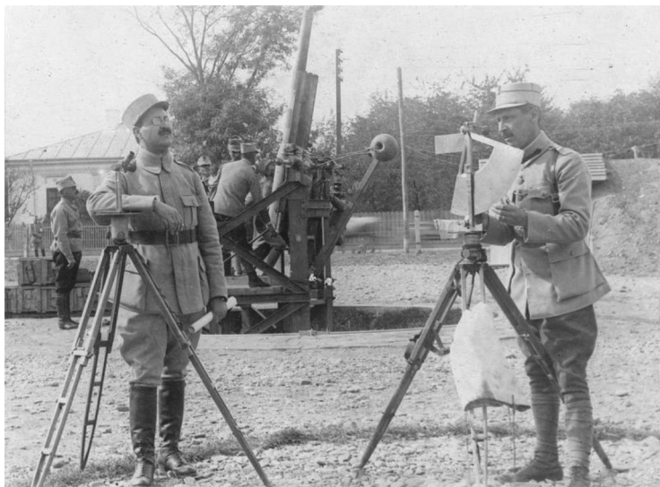
Photo 7: Romanian officers in the antiaircraft artillery and devices to establish the flight height, speed, and trajectory
