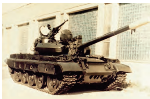
Figure no. 3: The modernised Phase II T-55 tank 30
